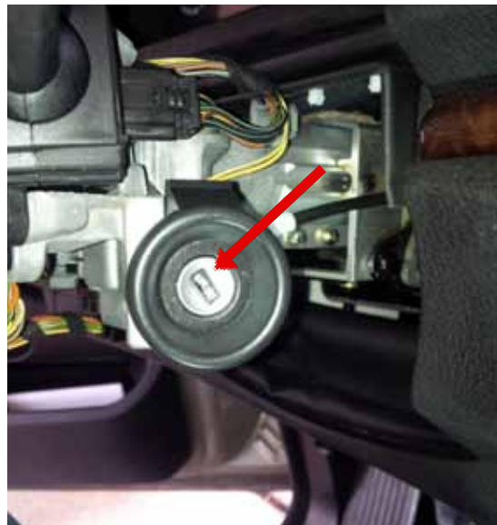
Figure 13 Key lock installed in housing with EWS ring (arrow shows release tool location)
