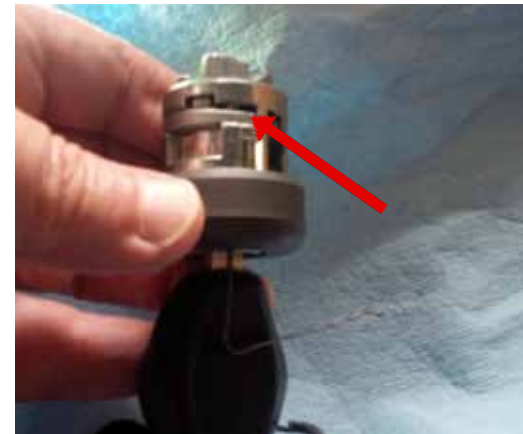
Figure 12 Practice with new lock to operate locking cam
