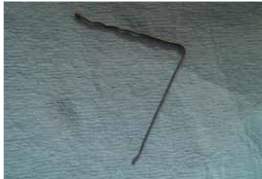
Figure 9 DIY "special" tool – copy the shape at the end and remove plastic
