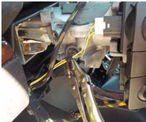
Figure 8 Small vise grips to pull and turn T pin
