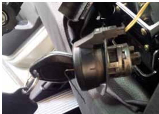
Figure 10 Key out with bobby pin holding cam latch down
