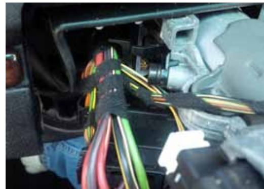
Figure 5 Switch wiring and upper retainer screw
