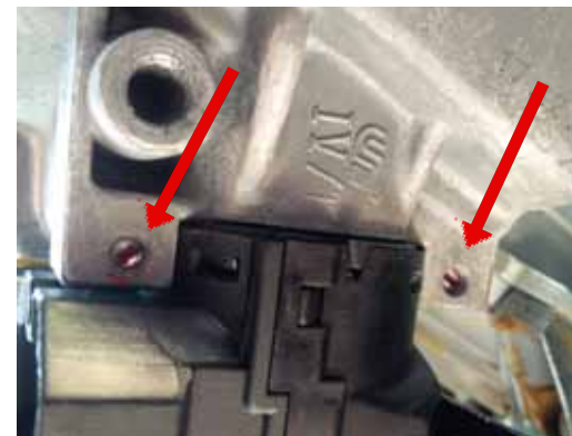
Figure 6 Set screws to hold switch
