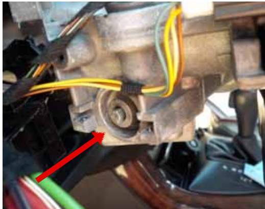
Figure 7 T shaped pin drives ignition switch
