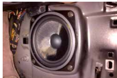
Figure 6 Installed BSW speaker
