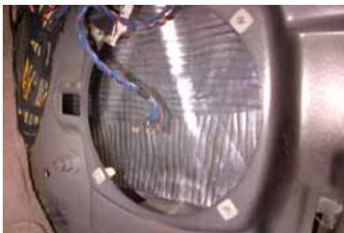
Figure 4 Installed Fatmat material
