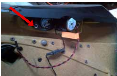
Figure 12 Tweeter mounting with washer
