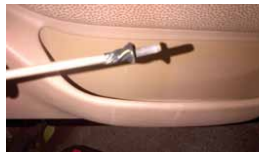
Figure 13 Torx screw retention for installation
