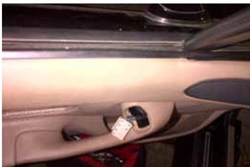
Figure 10 Mirror switch removed
