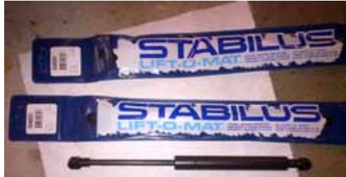
Figure 2 E53 Hood replacements
